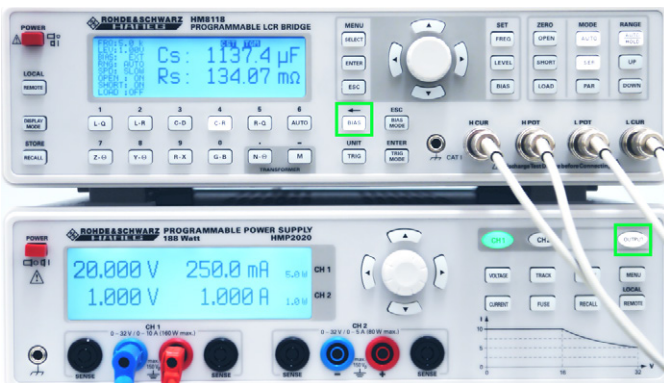
Fig. 7.6: Activate external BIAS preload
