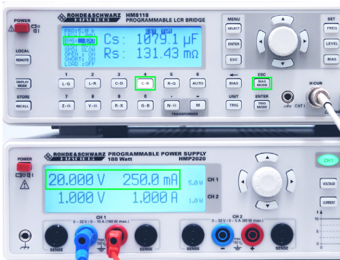
Fig. 7.5: Activate external BIAS preload
